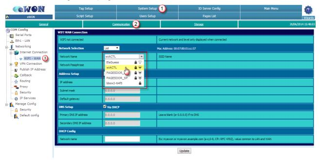
If the Wifi-card is present and correctly detected, the available networks in the range are shown in the drop-down field next to **Network Name**.
